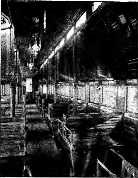
Fig. 152. INTERIOR OF TOURIST OR EMIGRANT SLEEPING CAR. SOUTHERN PACIFIC COMPANY. (Details shown in Figs. 505-511)
